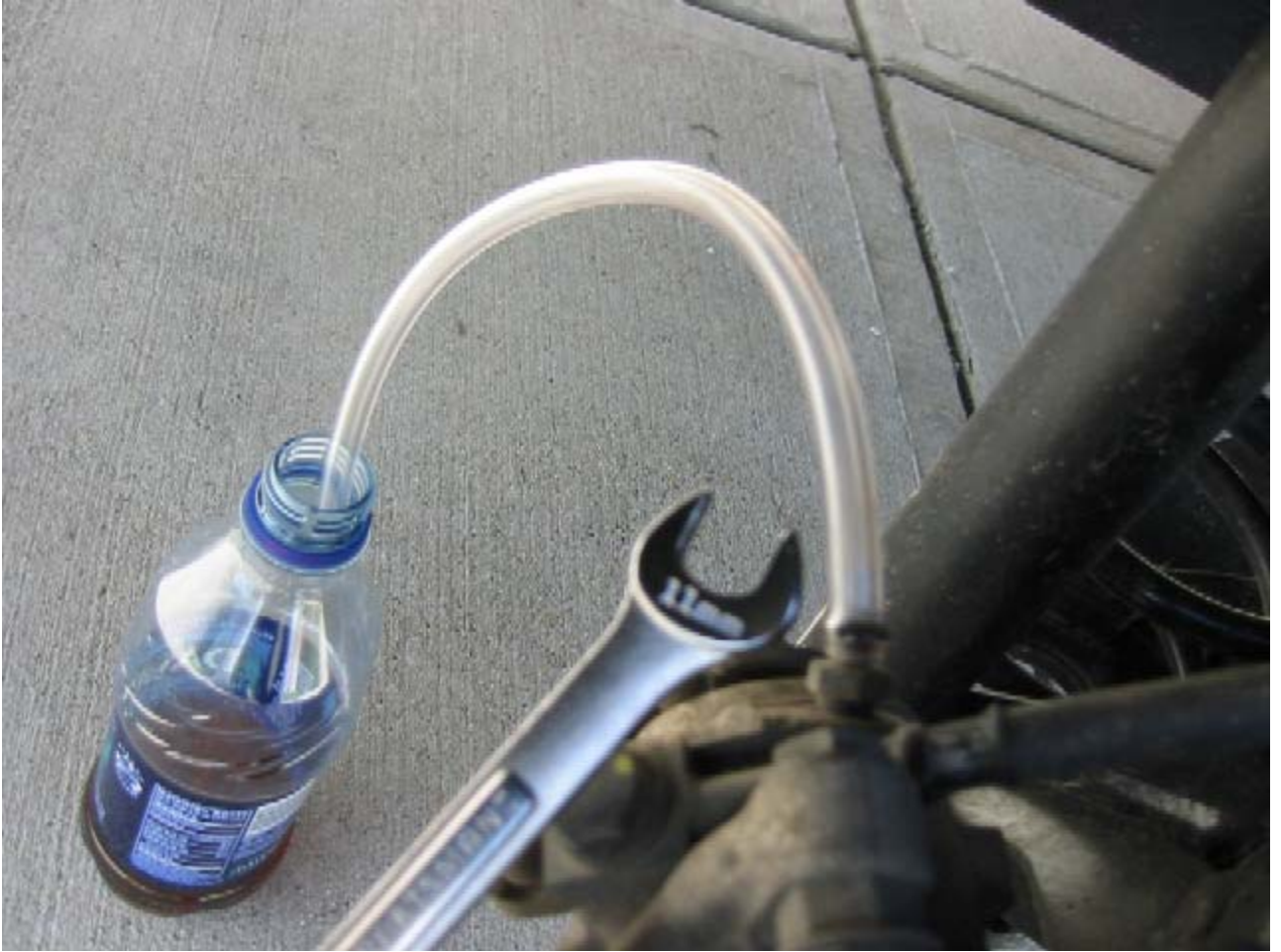
Bleeding out the amber fluid (note the rust bits which I think came from the screw area as they were only present after opening it up)
