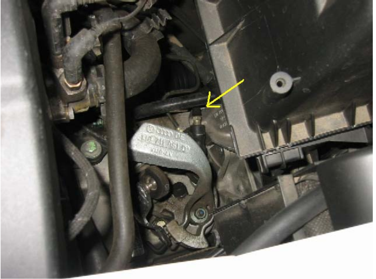
Motive bleeder connected to reservoir
