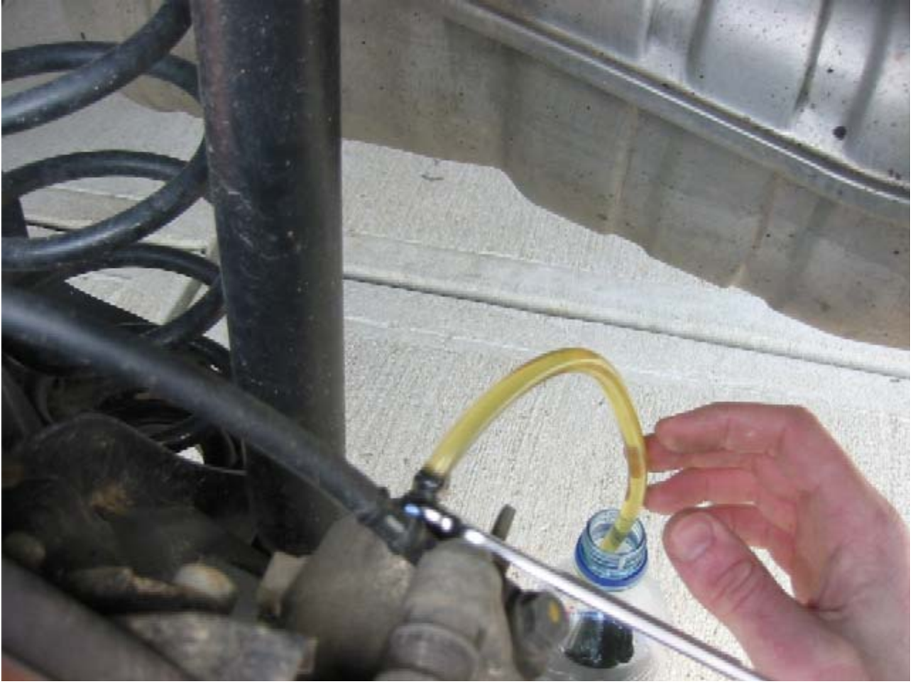
Blue fluid begins to show as a fine line in the center of the stream
