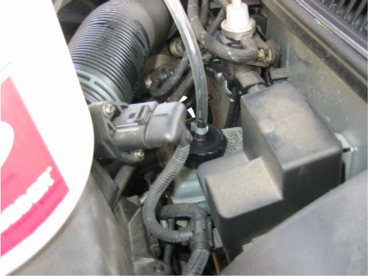
View of reservoir (NOTE the markings for min and max are to the right of the text and obscured in this pic)
