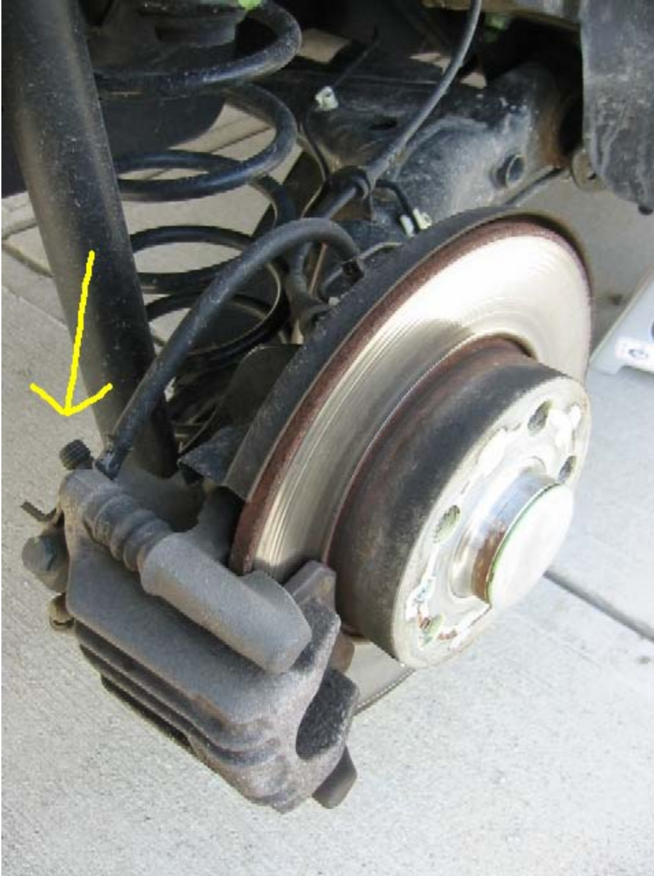
Left rear brakes (notice the pads are toasted!)
