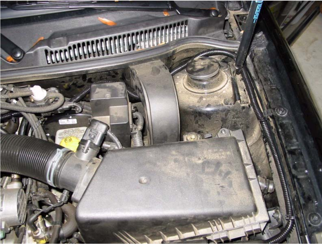
The wire loom is routed between the battery and the airbox, along the hood release cable, then over and along the rear edge of the engine compartment. It's zip-tied along the way to keep it in place. This is a good photo to show how much yellow pollen is in the air in Atlanta in the springtime!
