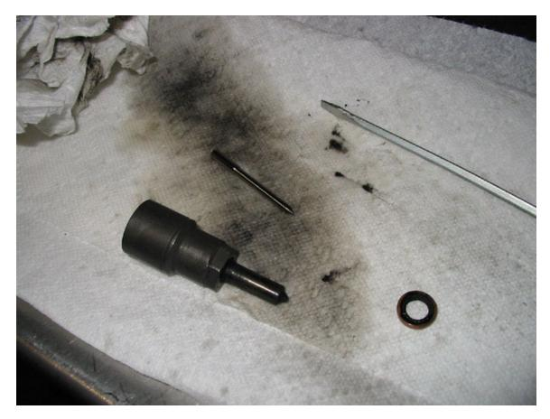
The washer can be a real pain to get off from around the base of the nozzle. Just be persistent. Soak the end in diesel/biodiesel, use the toothbrush, and use a small flat-blade screwdriver to scrape the soot out from the INSIDE of the washer surface. Try to rotate the nozzle against the retaining nut. Keep doing this until things start to come apart.
