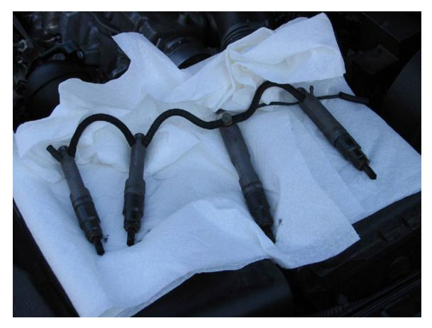
Here are the four injectors out of the engine, with the return lines still attached. All done! If you're swapping nozzles, continue on, but if not just go on to the installation part at the end.
