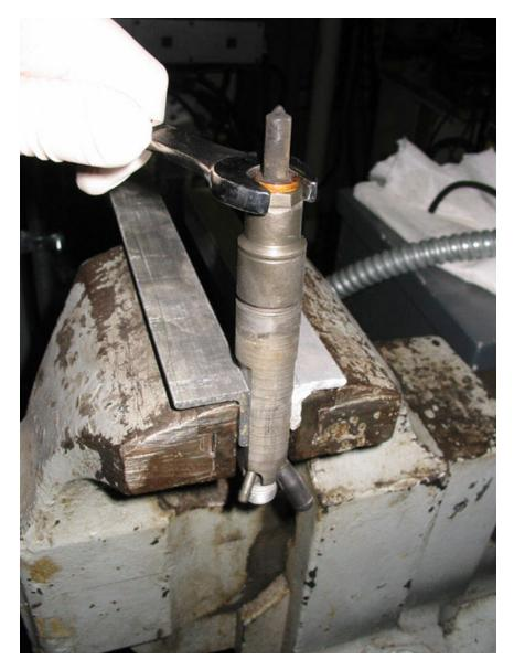
I cannot stress enough how helpful a vise is to have here. It keeps the injector stable, upright, and given that I had to use a cheater bar to crack two of the retaining nuts, allows for more leverage than you can get by using two wrenches.
