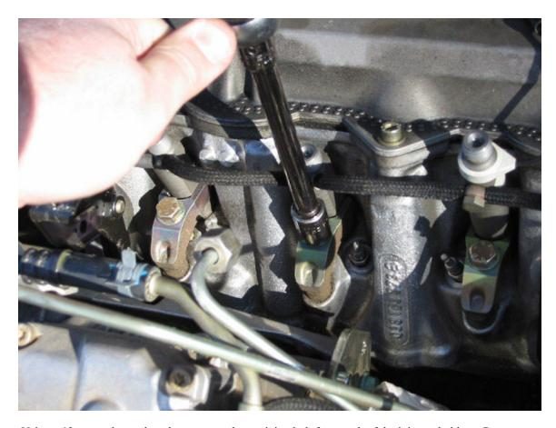
Using a 13mm socket and ratchet, remove the retaining bolt from each of the injector holders. Remove each holder, being careful not to drop the nut and the special washer.
