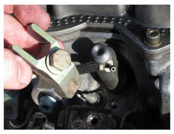
Here's one of the injector holders. Notice the crud buildup. I gave these a good cleaning along with the dimple in the head to make sure that the mating surfaces were clean on reinstall.
