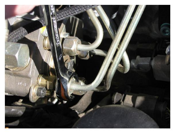
Use a 17mm flare-nut wrench (or your regular 17mm wrench) to crack the fuel lines at the pump. You won't take these off the pump, you'll just rotate the lines away from the injectors to get them out of the way, so just loosen the nuts about half a turn. You might want to put a towel underneath the pump to catch any drips. I didn't see any on mine, but there's lots of rubber underneath there, so it would be a good precaution.
