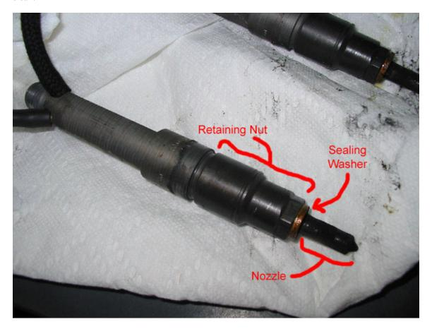
This is clearly a "before" photo of one of my injectors. What a mess! Notice all the soot caked on the nozzle. This soot has caked inside the sealing washer, which now won't come off. I removed the retaining nut and nozzle from the injector before trying to remove the sealing washer, but you can do that step first if you're so inclined.
